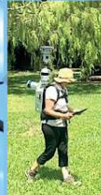
LiDAR - Measuring 3D structure of land and vegetation
